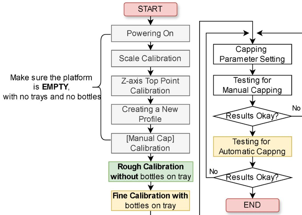
Note: After changing to a new bottle profile, large scale calibration and Z-axis top point calibration are optional.
