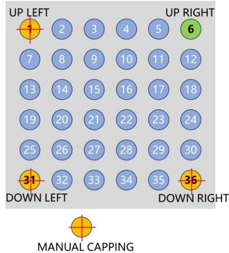
Note: The UP RIGHT position does not need calibration. This position will be automatically completed based on the UP LEFT, DOWN LEFT, and DOWN RIGHT three positions.
